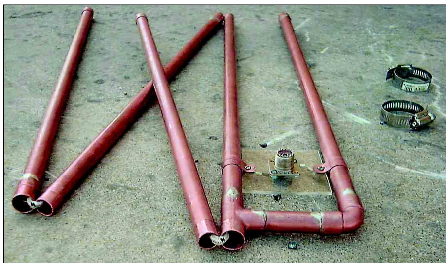
Figure 6—The J-pole in the process of being “folded.”
