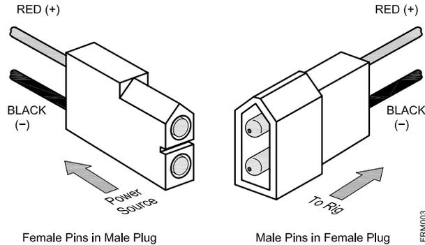
The 12-A Molex 1545 series connector (part numbers: male, 03-09-2022; female, 03-09-1022) is adequate for low power mobile radios, handhelds and accessories.
